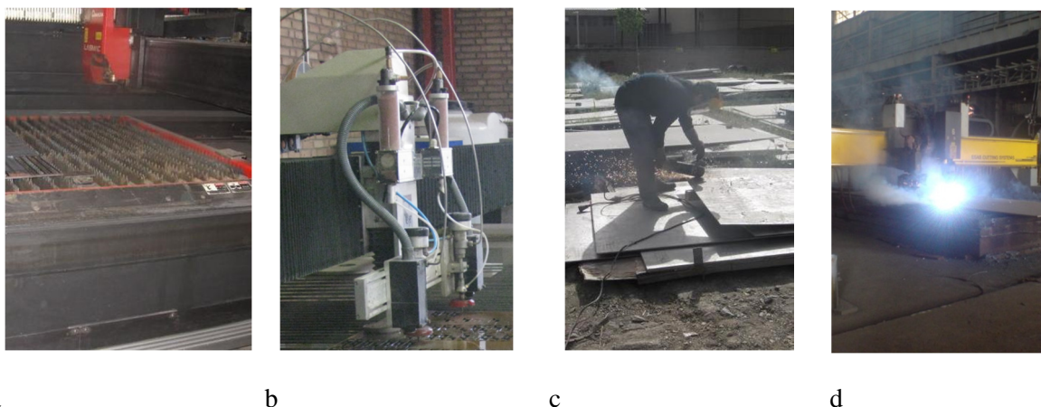
Figure 2 a) Used laser beam cutting machine b) Water jet setup c) Cutting by grinder wheel d) cutting by plasma arc machine
